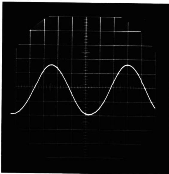
This unretouched photo shows the acoustic output of the system when driven by a 50 W sine wave signal at 35 Hz. A laboratory microphone was used to pick up the sound from the 4311B. The signal from the microphone was connected directly to an oscilloscope and the trace photographed.
